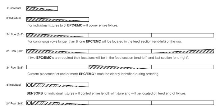
**SENSORS** for rows will control the feed section (end-left) of the row. Sensors can control more than an 8' section within a row. Consult factory for sensor/section options, or for multiple sensors in a continuous row.
