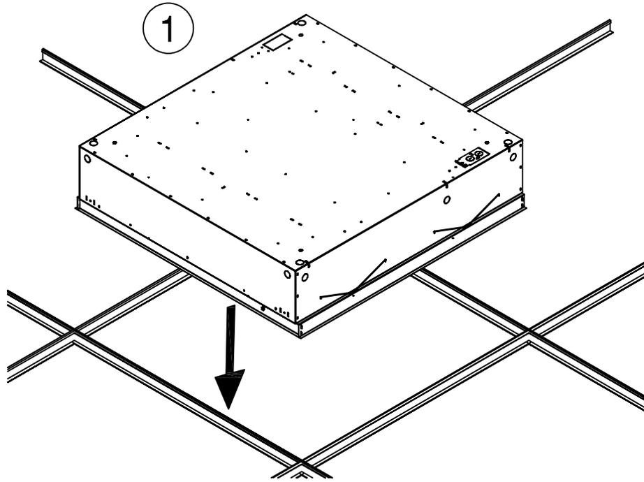
1. DROP FIXTURE INTO APPROPRIATE SIZED GRID OPENING FROM ABOVE GRID.
